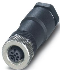
Power connector, 4-position, Socket straight M12, Coding: A, Screw connection, knurl material: Zinc die-cast, nickel-plated, cable gland Pg11, external cable diameter 8 mm ... 10 mm
