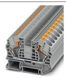
Feed-through terminal block, nom. voltage: 1000 V, nominal current: 76 A, connection method: Push-in connection, number of connections: 2, cross section: 0.5 mm² - 25 mm², AWG: 20 - 4, width: 12.2 mm, color: gray, mounting type: NS 35/7,5, NS 35/15
