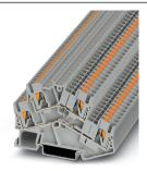
Double-level terminal block, connection method: Push-in connection, cross section: 0.14 mm<sup>2</sup> - 4 mm<sup>2</sup>, AWG: 26 - 12, width: 5.2 mm, color: gray, mounting type: NS 35/7,5, NS 35/15
