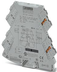
Configurable temperature transducer with plug-in connection technology for connecting 2, 3, and 4-conductor resistance thermometers and resistance-type sensors. Configurable via DIP switch or software. Screw connection technology, standard configuration
