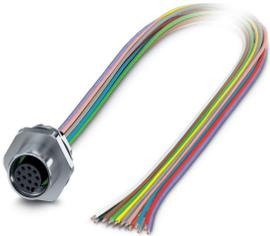
Flush-type connector, Universal, 8-position, Socket, M12, A-coded, Front mounting, M16 x 1.5, Individual wires, cable length: 0.5 m, 0.25 mm<sup>2</sup>, TPE litz wire
