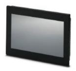
Touch panel with 25.9 cm / 10.2" TFT-display (analog resistive (polyester)), 16.7 million colors, Arm® Cortex®-A9, 1 GHz, 1x USB Host 2.0, 1 x Ethernet (10/100 Mbps), RJ45, Yocto/Linux and user software: Otter Browser. (bus system: without)
